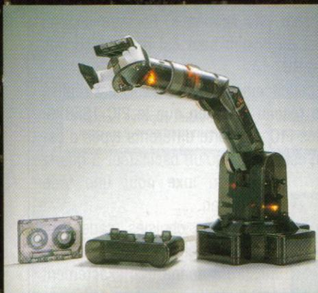
Robot Arm with programmable controller and software
