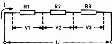
$$I = \frac{U}{R_1 + R_2 + R_3}, \quad \text{soit } I = \frac{U}{R}$$
